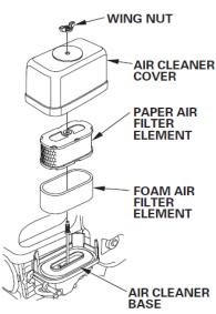
to remove dirt, or blow compressed air (not exceeding 207 kPa (2.1 kgf/cm2, 30 psi) through the filter element from the inside. Never try to brush off dirt; brushing will force dirt into the fibers.
