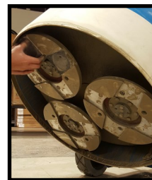
Underside - 3 gear drive heads with 4 metal plates per head
