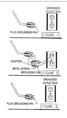
grounding pin is damaged or broken. The Green (or Green/Yellow) wire in the cord is the grounding wire. When replacing a plug, this wire must be attached to the grounding pin only. Extension cords connected to this machine should be 12 gauge, three wire cords with three prong plugs and outlets. DO NOT use extension cords more than 50 feet (15 m) long.
