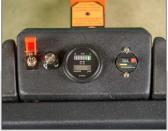
Simple to use control panel. Lift the safety toggle cover and simply flip the switch. Adjust the speed of the head assembly by turning the speed dial.
