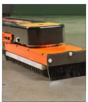
With the low profile pad driver the total height of the head assembly is 4 1/8 inches tall, allowing the user to get under even the tightest of spaces.
