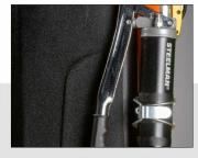
The only maintenance the machine really requires is greasing the head assembly. With the attached grease gun this reduces maintenance to just a few seconds.
