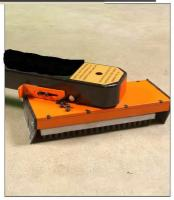
With the head locking feature the EdgeGlider head can literally self guide along a wall or edge, allowing for less user fatigue and ease of use.
