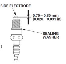
When installing a new spark plug, tighten 1/2 turn after the spark plug seats to compress the washer.
